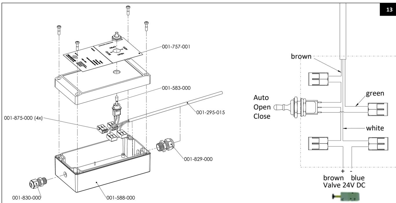
Wiring plan L'port & T'port FeedStation Walk-Through (control box art. no. 002-481-001). If the switch works the other way around, rotate it by 180 degrees.
