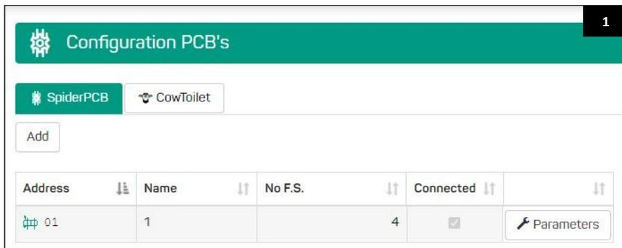
Select the SpiderPCB (fig. 1) to be configured. The screen will open as shown in figure 3. Select 'Add' if no SpiderPCB is displayed or if an additional one needs to be added. Then the next screen will open (figure 2). Select the number of feeding stations you want to add, as well as the number of feed types per feeding station. Select the motor type. Note: these are preconfigured settings and can be changed in the next screen. Once the selection has been made, click 'Apply'.
