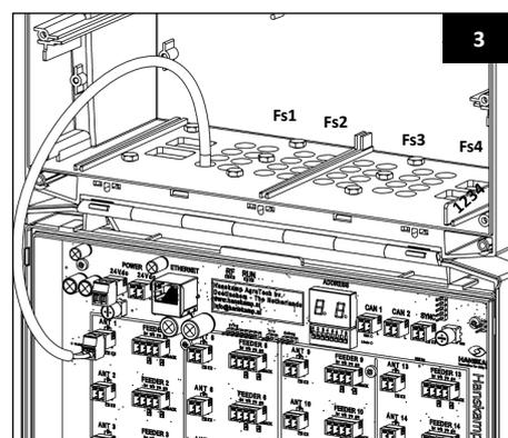
All inputs and outputs are numbered, as is the cable entry plate (art. no. 005-161-001) (fig. 3). Ensure that the holes line up with the inputs and outputs to keep the cables uncluttered.
