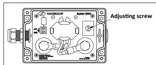
5. Tighten the adjusting screw in the EWA until the LED for the relevant Antenna flashes green. If the adjusting screw is fully tightened but the transponder is still not being identified, move the transponder further in. If it is recognised, the EWA is correctly adjusted.
