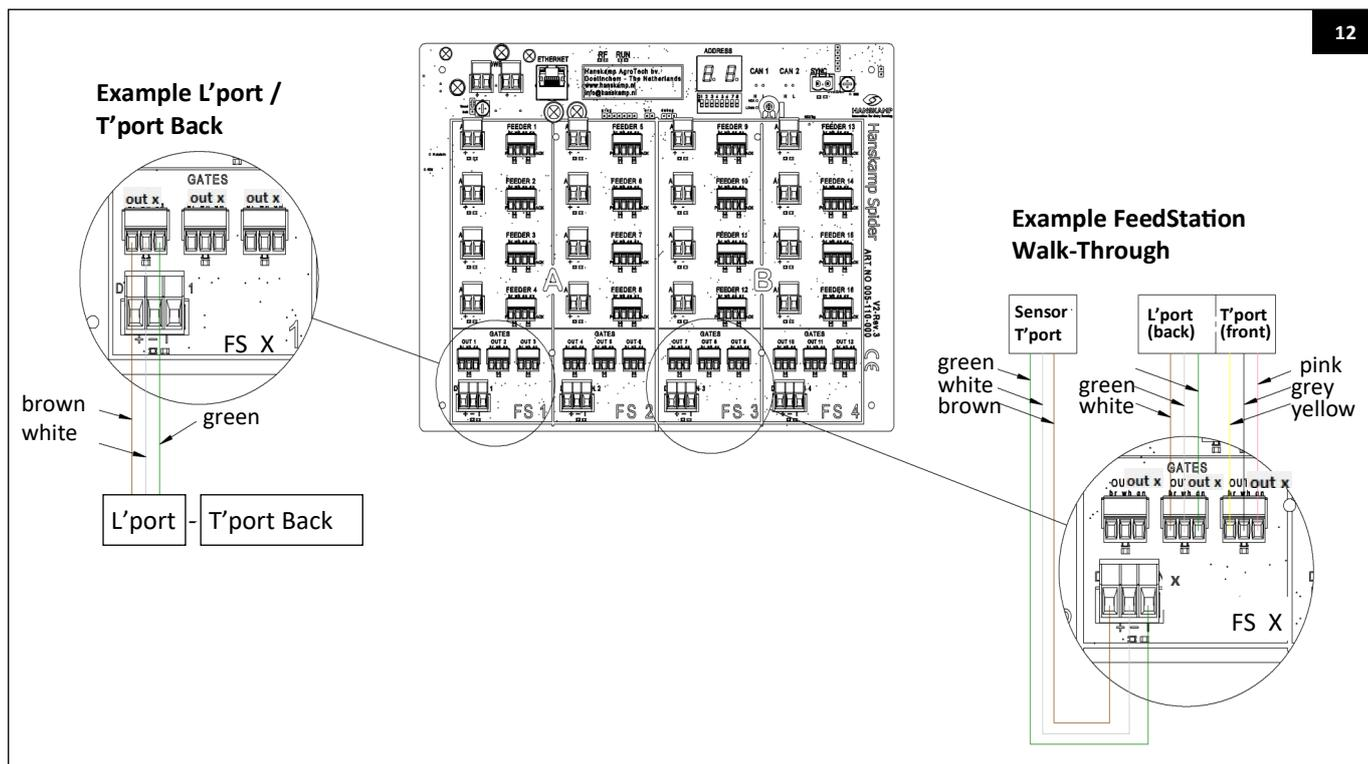
L'port connection diagram (control unit art. no. 002-480-001). If the switch works the other way around, rotate it by 180 degrees.
